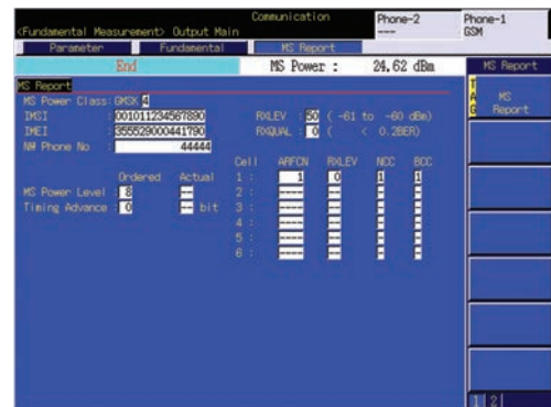
Mobile Terminal Report Monitor (GSM)
